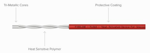
FyreLine linear fixed heat sensing cable is constructed using two twisted and tensioned, tri-metallic conductors. Each of the conductive cables are coated in a heat sensitive polymer which, when heated to its rated temperature, melts, causing the two cables to touch. The resulting short sends a signal to the fire alarm control panel, indicating that a fire (or excessive heat) has been detected. Once a fire has been detected the damaged length of cable is easily replaceable.
