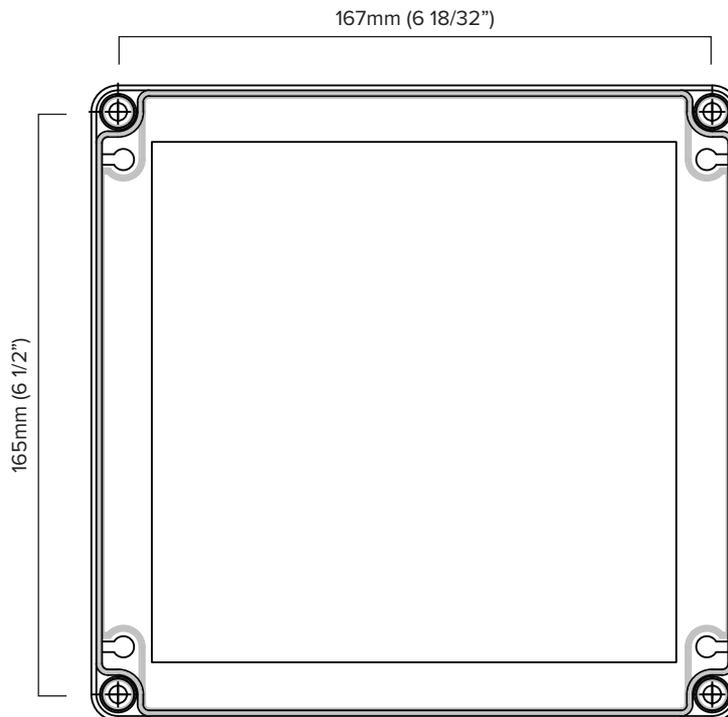
Figure 13: Fixing Dimensions for mounting FyreLine Analogue Heat Detector Controller
