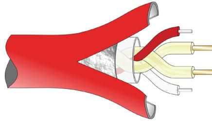
Figure 1: Analogue Linear Heat Detection Cable Construction
