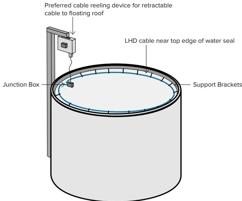
Figure 8: Typical locations for protecting floating roof storage tanks with LHD cable
