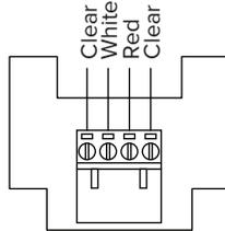
Figure 12: PCB Wiring Diagram
