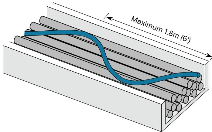
Figure 4: Sine wave pattern layout of LHD cable in a cable tray
