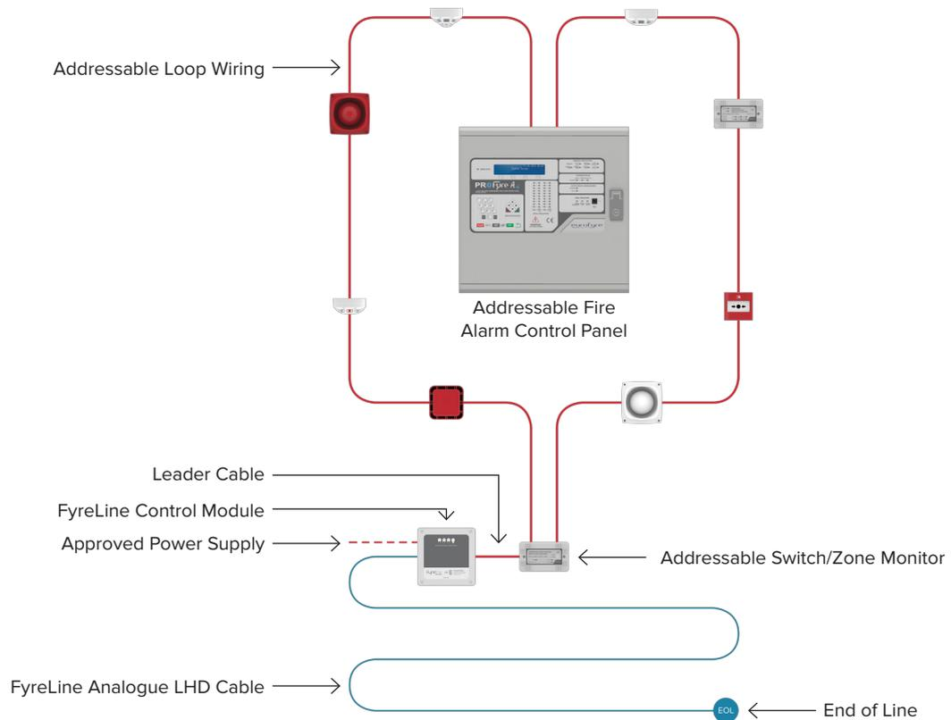
Figure 3: Typical Addressable System FyreLine Analogue Heat Detector Wiring Configuration
