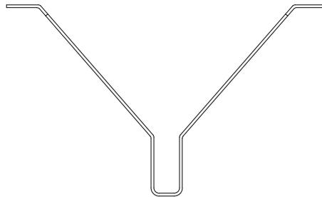
Figure 11: Typical “V” Bracket for supporting Linear Heat Detection cable
