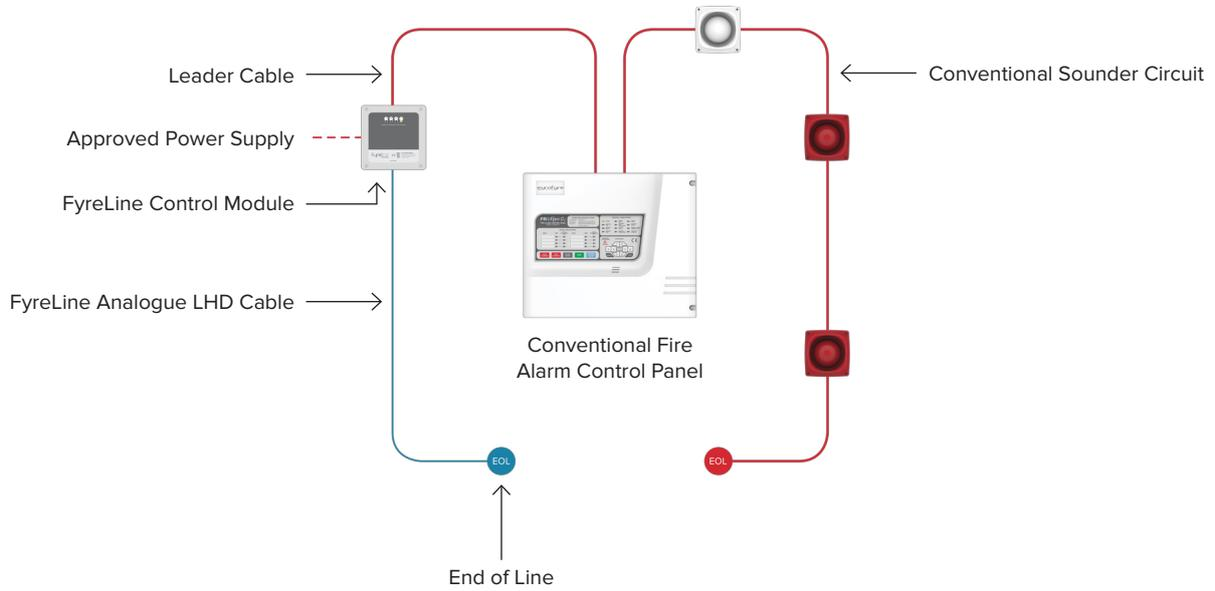
Figure 2: Typical Conventional System FyreLine Analogue Heat Detector Wiring Configuration
